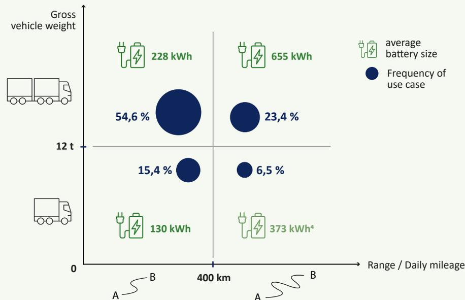
Snapshot of the percentages of medium-haul (up to 400 km) and long-haul transport and their distribution on medium-weight (up to 12 metric tons) and heavy-weight (above 12 metric tons) vehicles. The battery sizes of each quadrant were averaged based on the manufacturers' data.
